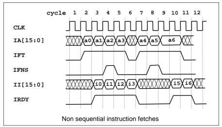
In systems with no instruction fetch wait states, e.g. with a synchronous instruction memory directly connected output IFNS can be ignored. In systems with wait states e.g. with an instruction cache or with debug access to the instruction memory IFNS must be used to abort pending fetches.
