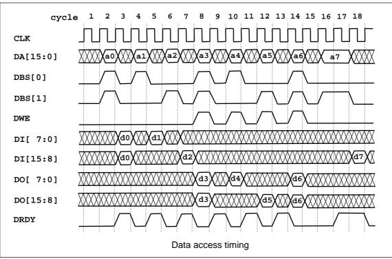
The second effect is the bus pipelining. Although the maximum access rate is one access every two cycles the bus is still pipelined as shown in cycles 17 and 18 where two accesses are completed in two consecutive cycles.
