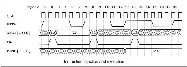
A type 2 example starts in cycle 8 where opcode **i1** is injected. When **STPD** is re-asserted in cycle 13 the destination operand **d1** is available at **DBGO[15:0]**. The example shows the behavior of an mtdp
